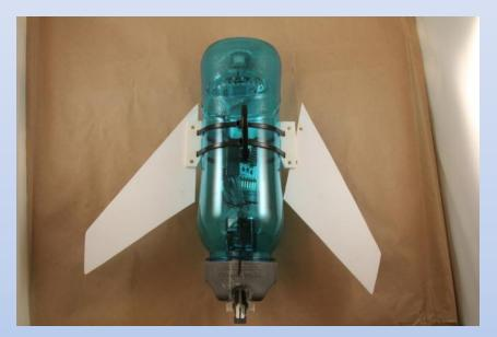
Place wings in wing yoke and mark the holes with a pencil.
